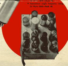
This amplifier operates very nearly Class B with relatively small current flowing in the final tubes without input signal. The wide frequency range, the low distortion, the low equivalent generator impedance, together with the high efficiency, permit a wide variety of applications, among which are the following:
