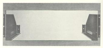
Slide the instrument in until it stops at the adjust position latches. Press the latches in and continue to slide the instrument until its front panel is flush with the cabinet panel.
