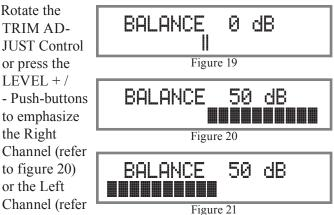
The Front Panel Display indicates the Balance changes in steps from 0 to 50dB. After approximately 3 seconds the Information Display returns to indicate the Source Selection and Volume Level. When the Balance is set to favor either left or right channel, the volume number indicated will have a "< or >" symbol on either side of the number.
