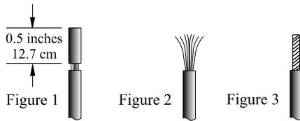
Note: If desired, the twisted ends can be tinned with solder to keep the strands together, or attach spade lug and/or banana connector.
