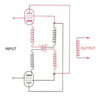
Fig. 2—Representation of McIntosh output circuit.
