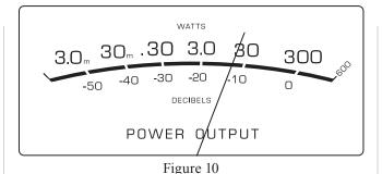
Watts- The meters respond to all the musical information being produced by the amplifier. They indicate to an accuracy of at least 95% of the power output with only a single cycle of a 2000Hz tone burst.
