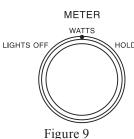
Note: When Power Control Input of the MC302 is connected to a Audio Preamplifier or A/V Control Center with Remote Meter Illumination Control, the Meter Illumination will automatically be remotely controlled (On/Off) with the METER Switch set to the WATTS or HOLD position.
