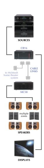
All it takes is one cable to join the CR16 and the MC58 (or MC7108) ... and one more to link a multizone system to a home theater.
