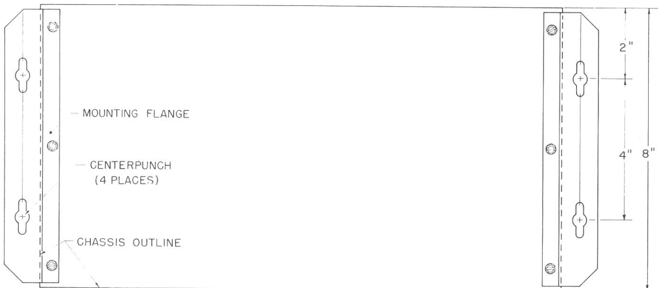
Figure 4. Bottom of MC75 with mounting flanges attached
