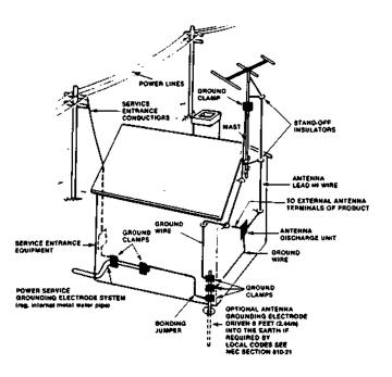
14. Outdoor Antenna Grounding - If an outdoor antenna is connected to the antenna terminal, be sure the antenna system is grounded so as to provide some protection against voltage surges and built up static charges.
