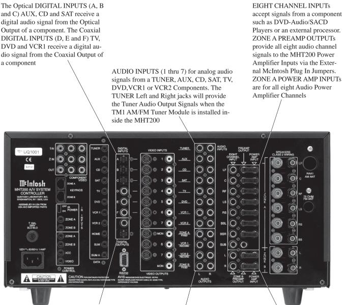
DIGITAL OUTPUTS both optical and coaxial, provide a digital audio signal to an external digital processor ZONE B PREAMP OUTPUTs provide Left and Right Channel Audio Signals to the MHT200 Power Amplifier Inputs via the External McIntosh Plug-In Jumpers. ZONE B POWER AMP INPUTs are for both Audio Power Amplifier Channels
