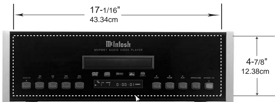
MVP861 Front Panel Custom Cabinet Cutout
