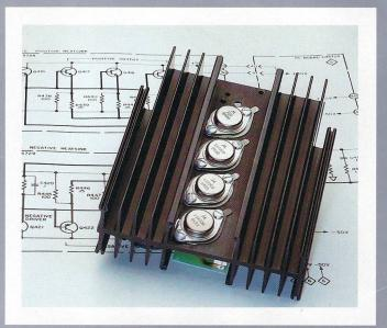
McIntosh cool operation requires a combination of careful design of the output circuit, containing the output circuit in a mechanical housing that permits the use of generous sized heat sinks to provide great heat dissipation capability along with chassis construction that permits adequate ventilation, then correctly matching the cool operating output circuit to the loudspeakers with a McIntosh designed and manufactured auto-transformer.
